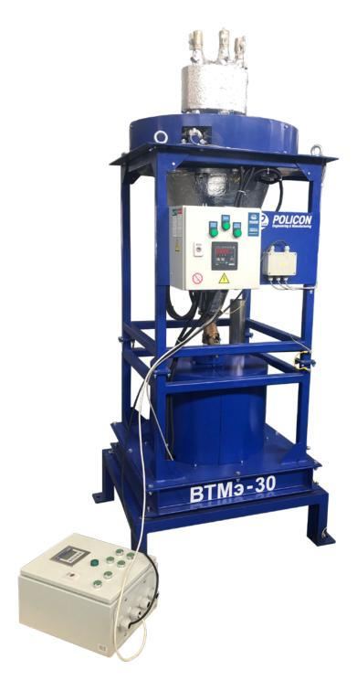
Tensometric hopper weigher consisting of a body mounted on a frame fixed to the overpass through anti-vibration supports. A ladle and an intermediate container are placed inside the body. Ladle, intermediate tank, feeder elements in contact with the product are made of stainless steel.
